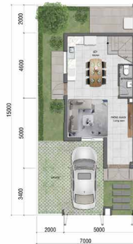
TẦNG TRỆT GROUND FLOOR
